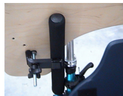
pic. 26: tubular armrest mounting
