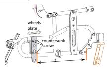
pic. 10: Displacement of the posterior wheels plate
