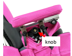
pic. 6: hip guide depth/height adjustment
