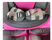
pic. 13: pelvic belt adjustment
